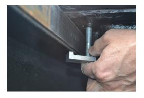
3. Remove clamp from the tonneau side of the toolbox frame
