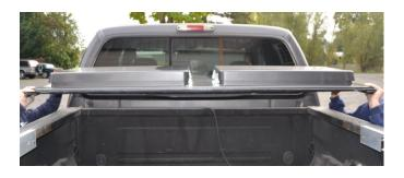
6. Using two people lift the toolbox frame off of the pickup bed.
