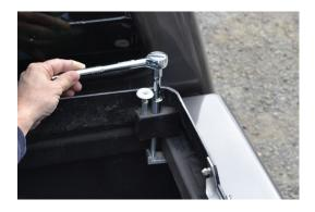
5. Remove the 3/8" bolts from the cab end of the toolbox frame
