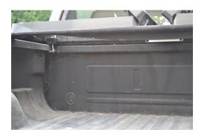
4. Slightly elevate the toolbox frame and slide the toolbox out.
