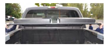
6. Using two people lift the toolbox frame off of the pickup bed.
