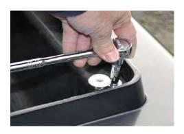
2. Remove 3/8" bolts from the tonneau side of the toolbox frame
