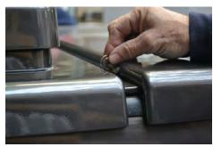
2. Close the tonneau back down, remove clips from both sides.
