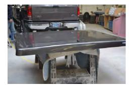
4. Place the tonneau on a flat surface while not on the truck.
