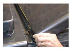
3. Using two people, lift the tonneau cover off of the male hinge.
