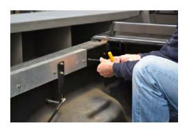
1. Remove the ¼" bolts from the male bracket and remove the bracket.
