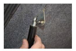
1. Hold the tonneau in the open position and remove the female strut end from the male ball stud end on the tonneau bracket. Repeat on the other side.
